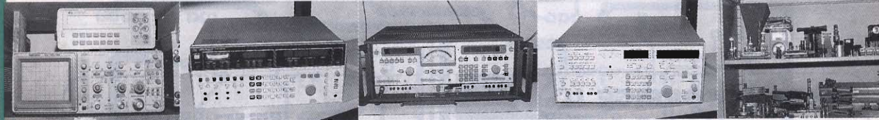
TEK2235 100 MHz oscilloscope HP 3468 DMM HP 3586 B Selective level meter HPIB W.G. SPM 19 selective level meter HPIB ANRITSU ML422B selective level meter HPIB Accessori microonde a stock
